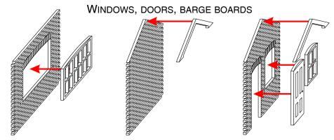
CUT ALL OF THE WINDOWS, DOORS, AND BARGE BOARDS OUT OF THEIR FRETS. APPLY A LITTLE BIT OF GLUE ON THE EDGE OF THE WINDOW OR DOOR AND PUSH IT INTO THE OPENING. IT IS RECOMMENDED TO PUSH THEM IN FROM THE BACK TO AVOID ANY GLUE MARKING THE COLOURED BRICKWORK. GLUE THE BARGE BOARDS FLUSH WITH THE SLOPED EDGE OF SIDES. CARE HAS BEEN TAKEN TO MAKE SURE EVERYTHING FITS WELL BUT SOME PARTS MAY FIT VERY SNUGLY. IN THAT CASE USE GENTLE PRESSURE TO PUSH THE PARTS INTO THE OPENINGS.
