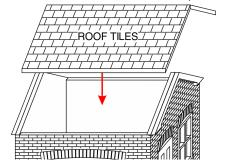
GLUE THE ROOF TILE PANELS TO THE BUILD-ING MAKING SURE THAT THEY ARE ALL EVEN ON ALL SIDES AND THERE IS NO GAP ON THE TOP RIDGE.
